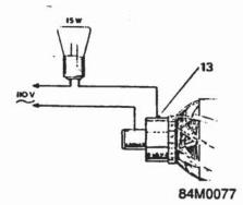
Test the armature for insulation and open or short circuits. Use a test lamp (110 volts, 15 watts). Renew if the armature if faulty.
