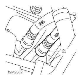
**2.** Release quick fit connector and disconnect fuel feed hose from fuel pipe.
