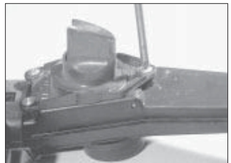
3.12 Removing the air cleaner intake duct adapter
