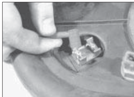
3.9 Disconnecting the vacuum pipe from the thermac valve
