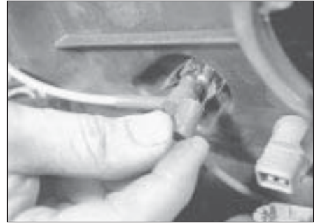
2.2b . . . and the thermac valve vacuum pipe
